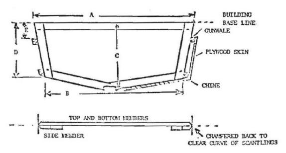
Note: It will be seen that the plywood is in contact with the moulding frames at the bottom but not the sides.
